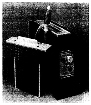
(25°C), RESIST STRIP (45°C) or IMMERSE TIN (21°C) . **Neons** indicate when the mains heater is operative. Supplied complete with syphon, IEC socket metre mains and 2 cable with moulded 13amp plug.
